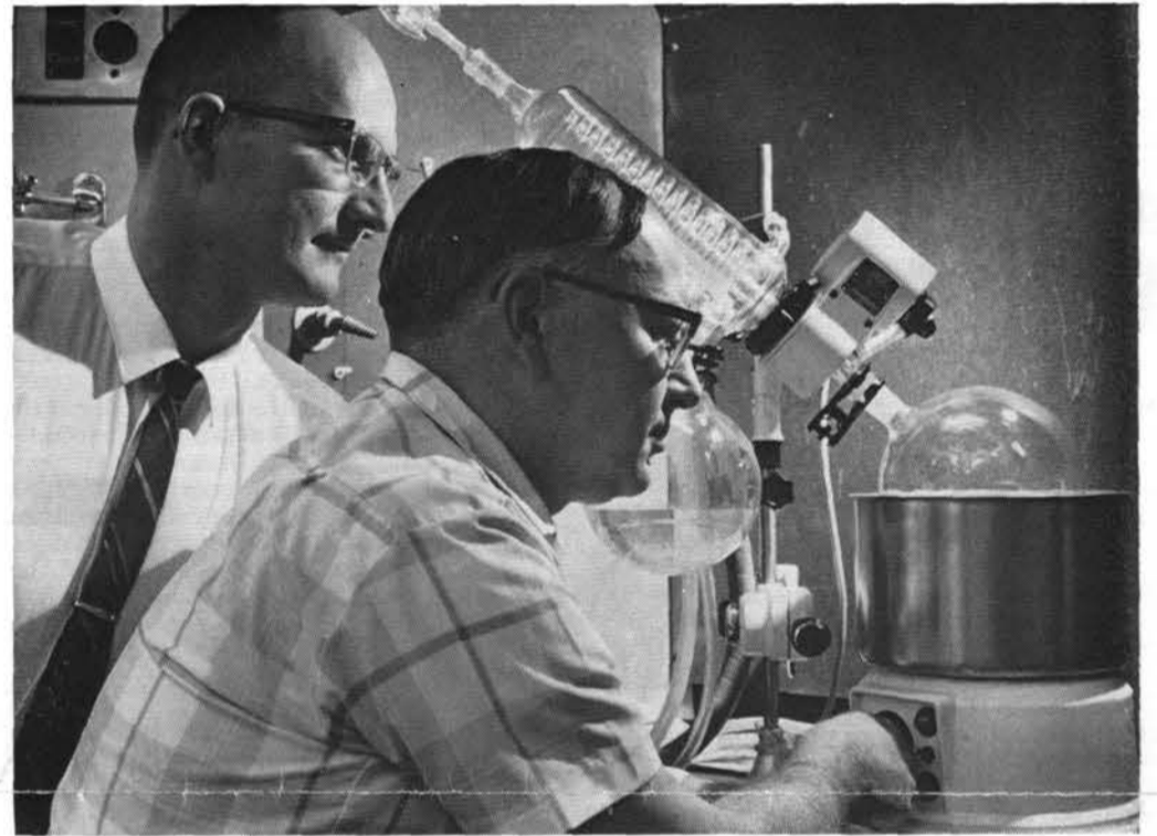
BUBBLE MACHINE? No, it's a rotary evaporator used to concentrate pre-ceramic materials in a ferroelectric ceramics process. Developers of the process, are, left, Paul Wilcox and Jim Hesse (both 2317).
